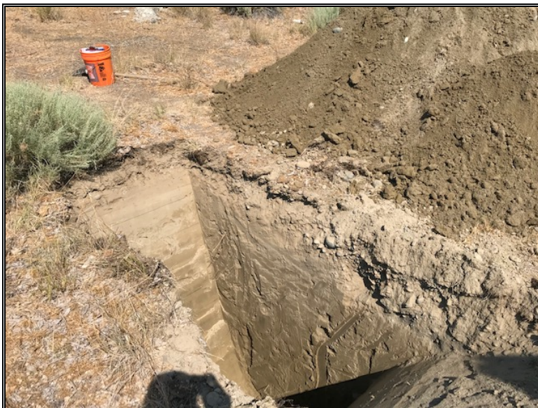
Exposed subsurface soil profile within test pit TP-1
