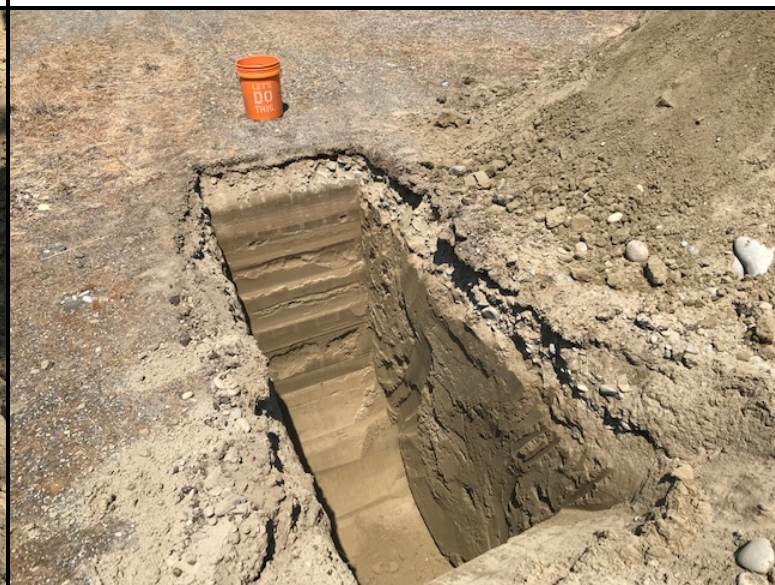
Exposed subsurface soil profile within test pit TP-8
