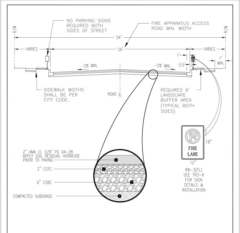
PERMISSIVE USE CASE: USE OF THIS NARROW STREET SECTION IS PERMITTED ONLY IN R-2S AND R-3 ZONED BLOCKS WHERE AVERAGE LOT WIDTH IS 40 FT OR LESS AND ADEQUATE OFF-STREET PARKING IS PROVIDED, OR AS APPROVED BY THE CITY ENGINEER.
