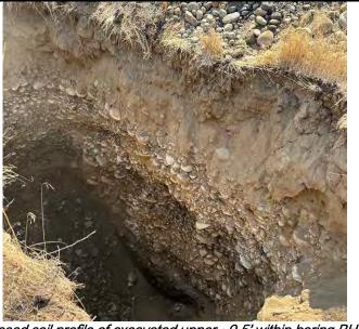
Exposed soil profile of excavated upper ~9.5' within boring BH-37
