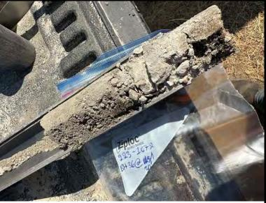
Soil sample obtained from boring BH-36 from 30' BGS
