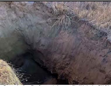
Exposed soil profile of excavated upper ~9' within boring BH-21
