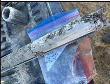
Soil sample obtained from boring BH-39 from 10' BGS
