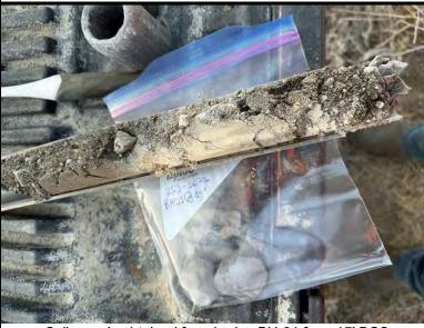
Soil sample obtained from boring BH-21 from 15' BGS
