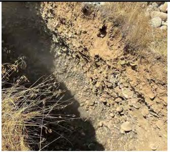
Exposed soil profile of excavated upper 9' within boring BH-41
