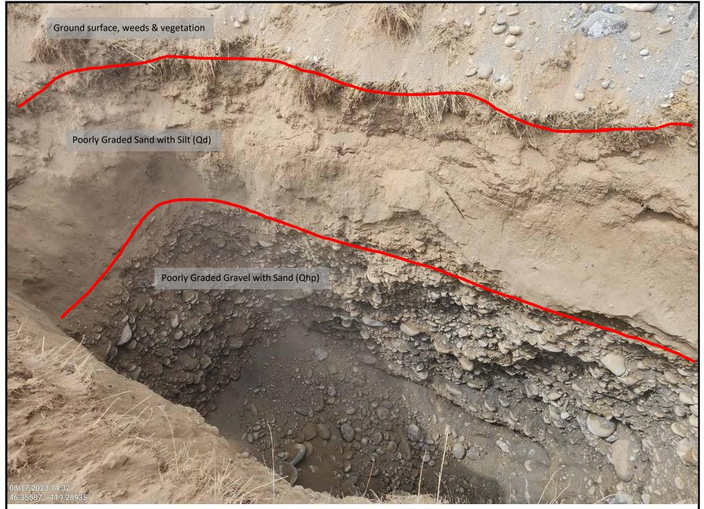
PLATE 20: SUBSURFACE SOIL PROFILE FROM UPPER ~11' OF BORING BH-20
