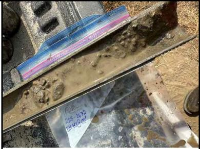
Soil sample obtained from boring BH-40 from 65' BGS
