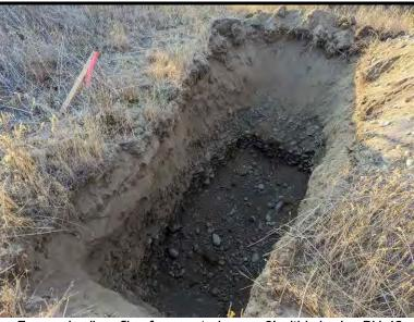
Exposed soil profile of excavated upper 8' within boring BH-42
