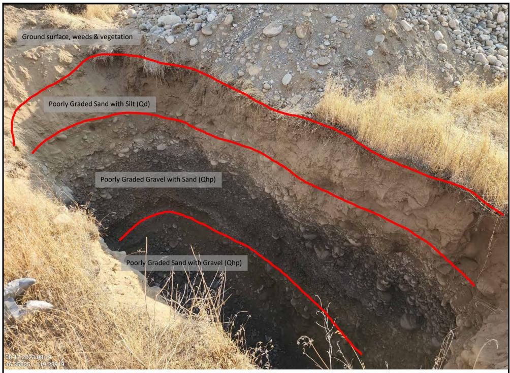
PLATE 19: SUBSURFACE SOIL PROFILE FROM UPPER ~9' OF BORING BH-16
