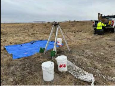
Down-hole seismic testing within boring BH-22 (DH-22)
