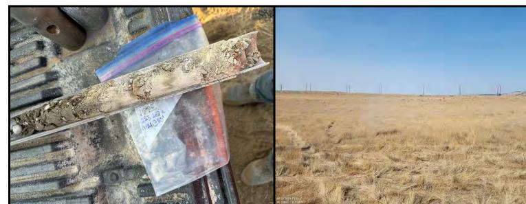
Soil sample obtained from boring BH-24 from 25' BGS
