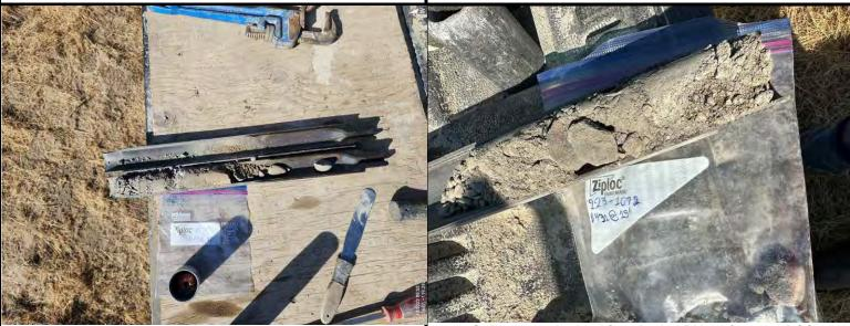
Soil sample obtained from boring BH-29 from 20' BGS
