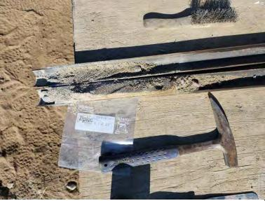
Soil sample obtained from boring BH-07 from 25' BGS
