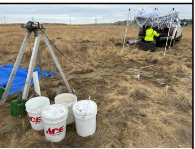
Down-hole seismic testing within boring BH-23 (DH-23)
