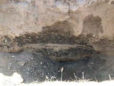
Subsurface soil profile within test-pit TP-4 / IT-2
