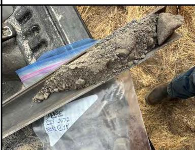
Soil sample obtained from boring BH-41 from 15' BGS
