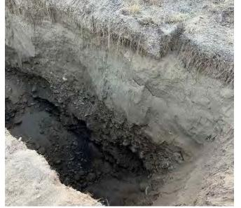
Exposed soil profile of excavated upper 9' within boring BH+PZ-40
