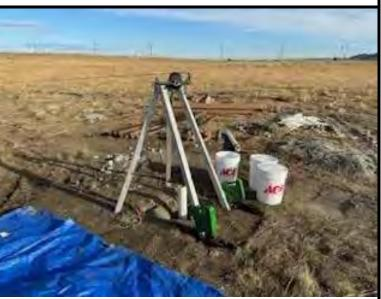
Down-hole seismic testing within boring BH-25 (DH-25)
