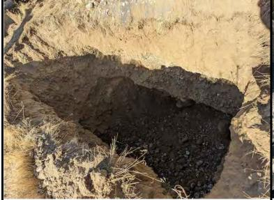
Exposed soil profile of excavated upper ~10' within boring BH-35
