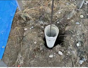
Down-hole seismic testing within boring BH-22 (DH-22)
