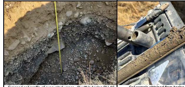
Exposed soil profile of excavated upper ~9' within boring BH-16
