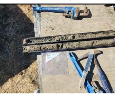
Soil sample obtained from boring BH-05 from 35' BGS
