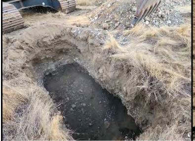
Exposed soil profile of excavated upper ~9' within boring BH-07
