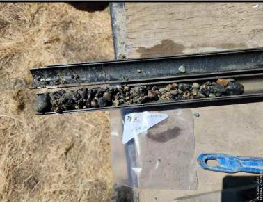
Soil sample obtained from boring BH-06 from 30' BGS
