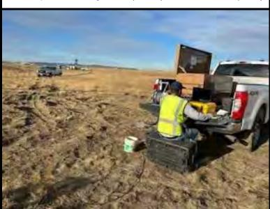
Down-hole seismic testing within boring BH-25 (DH-25)
