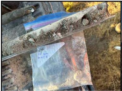
Soil sample obtained from boring BH-26 from 10' BGS
