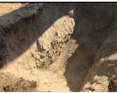
Subsurface soil profile within test-pit TP-9 / IT-4
