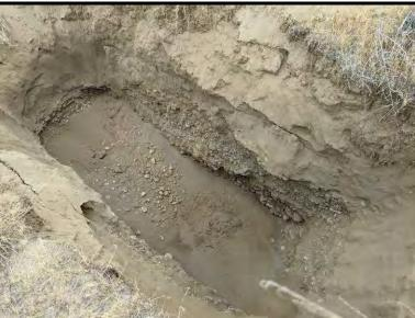
Exposed soil profile of excavated upper ~9' within boring BH-34
