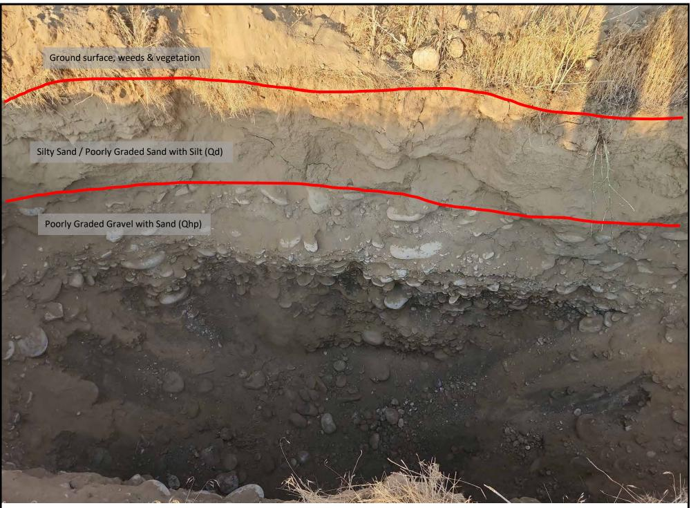
PLATE 18: SUBSURFACE SOIL PROFILE FROM UPPER ~9' OF BORING BH-12
