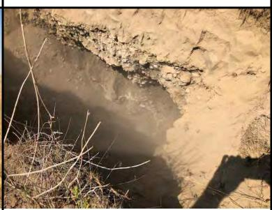
Subsurface soil profile within test-pit TP-3 / IT-1
