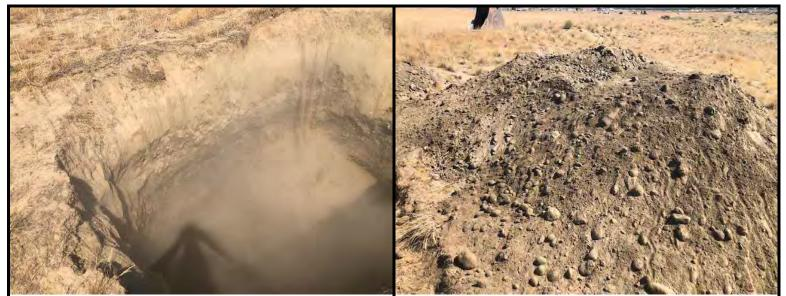
Subsurface soil profile within test-pit TP-2
