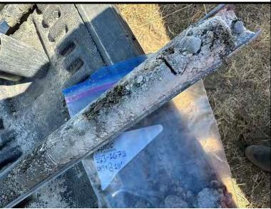
Soil sample obtained from boring BH-39 from 15' BGS
