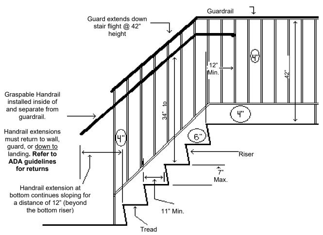
Graspable handrails at **34" to 38"** shall occur on both sides of the stairway (graspable details on reverse of this sheet).
