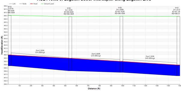
**HGL Profile of Logston Sewer Interceptor along Logston Blvd**
