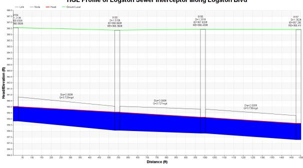
**HGL Profile of Logston Sewer Interceptor along Logston Blvd**
