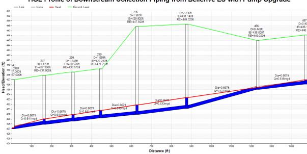
HGL Profile of Downstream Collection Piping from Bellerive LS with Pump Upgrade
